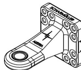
When using the drawbar eye on rigid drawbar trailers it should also be noted that the correlation between the height of the centre of gravity and the effective length of the drawbar (distance between centre of coupling and centre of axle or axle unit) with a permitted total mass of the trailer may not exceed 0,4.
