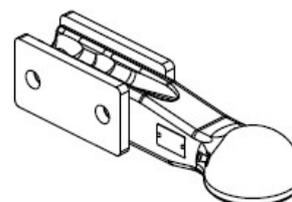
When using the coupling heads 80 on rigid drawbar trailers it should also be noted that the correlation between the height of the centre of gravity and the effective length of the drawbar (distance between centre of coupling and centre of axle or axle unit) with a permitted total mass of the trailer may not exceed 0,4.
